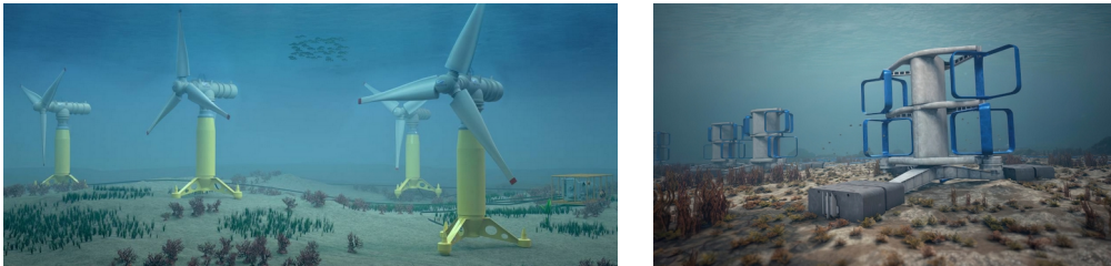
Normandie Hydroliennes project (on the left) and FloWatt project (on the right), based on the two main types of technologies: horizontal and vertical axis turbines, for a deployment in the Raz Blanchard
