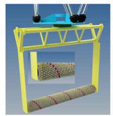
Experimental tests will be carried out in the wave and current flume tank of Ifremer, under a specified set of load cases (forced oscillations, current). These trials serve to assess the hydrodynamic loads acting on the cylinder.
