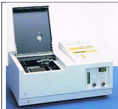
Figure 1.8a. Iatroscan MK6 used to analyze lipid classes
