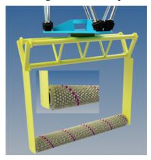
Experimental tests will be carried out in the wave and current flume tank of Ifremer, under a specified set of load cases (forced oscillations, current). These trials serve to assess the hydrodynamic loads acting on the cylinder.
